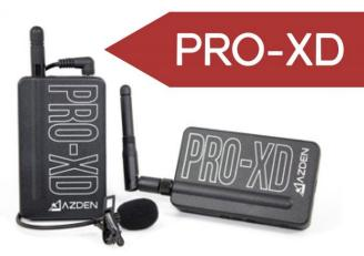
When you need to capture the voice or sound of a subject from further away, you need a wireless microphone. The PRO-XD is a digital wireless microphone system that can transmit better than CD quality audio to the receiver up to 35 meters away. It operates on the 2.4 GHz frequency band which is legal and license-free worldwide. The PRO-XD is priced so competitively that no one can come even close. Azden is the only brand that offers a quality digital wireless solution at this price point.
